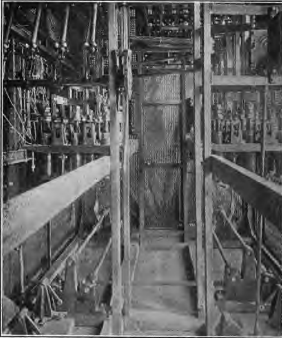
FIG. 71.—U. S. S. New Mexico : Interior View of Control Cell for Ship's Propelling Machinery
